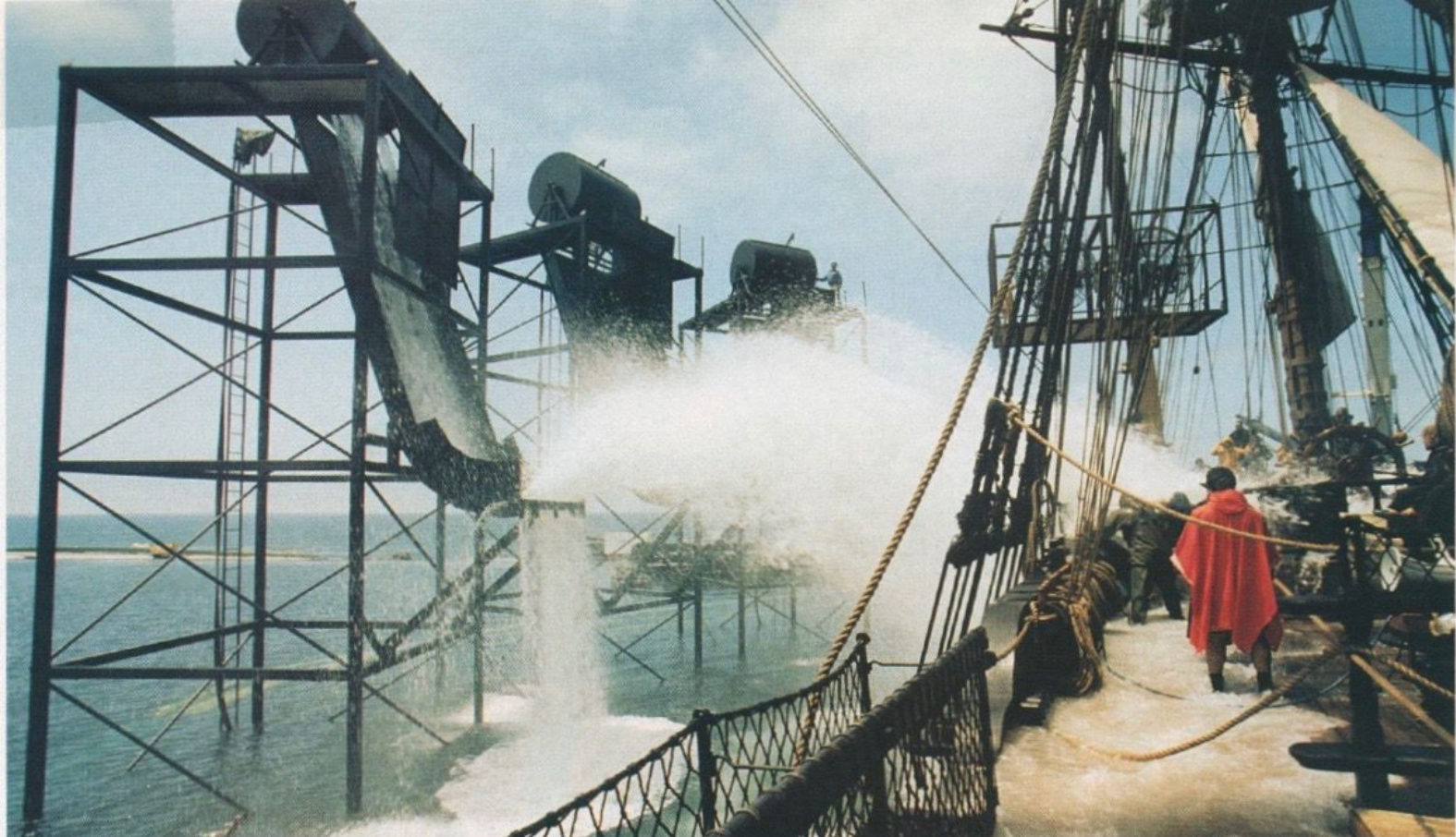
WEIR SCIENCE: Above, the Surprise gets pummeled by a gale-force storm, which the special-effects crew created with the help of two jet engines, wave and wind machines, and four dump tanks, each capable of dropping 3,000 gallons of water. "The dump tanks did throw people off the ship on occasion," Boyd says. "Luckily, I was the helmsman, so I was holding onto the wheel for dear life. No acting required." Left, Weir and Crowe work out a master plan.
